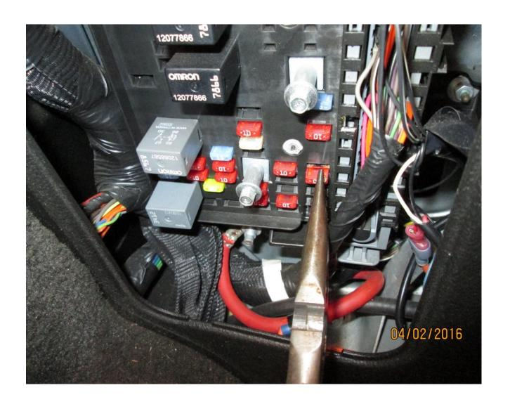
Replace with 1amp fuse or 2amp fuse.
